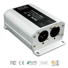
Artnet-DMX converter is the Ethernet Control System based on the Artnet protocol, used to convert the Artnet network data package into DMX512 data, adopting high-speed ARM processor, stable and reliable working. Following Artnet standard protocol, it supports RJ45 network interface and standard DMX512 output interface.
